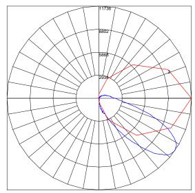
$\label{eq:maximum} \begin{array}{ll} \text{Maximum Candela} = 11736 & \text{Located At Horizontal Angle} = 00, \text{Vertical Angle} = 55 \\ \# \ 1 - \text{Vertical Plane Through Horizontal Angles (0 - 180) (Through Max. Cd.)} \\ \# \ 2 - \text{Horizontal Cone Through Vertical Angle (55) (Through Max. Cd.)} \\ \end{array}$
