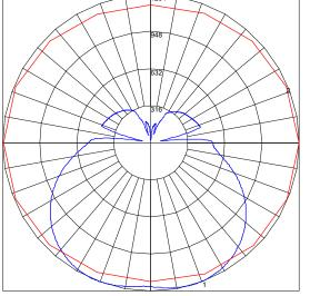
Maximum Candela = 1264.2 Located At Horizontal Angle = 0, Vertical Angle = 16.5 # 1 - Vertical Plane Through Horizontal Angles (0 - 180) (Through Max. Cd.) # 2 - Horizontal Cone Through Vertical Angle (16.5) (Through Max. Cd.)
