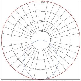
$\label{eq:maximum Candela = 5899.884 Located At Horizontal Angle = 90, Vertical Angle = 2 \ \# \ 1 - Vertical Plane Through Horizontal Angles (90 - 270) (Through Max. Cd.) \ \# \ 2 - Horizontal Cone Through Vertical Angle (2) (Through Max. Cd.)}$
