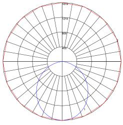
$\label{eq:maximum} \begin{array}{ll} \text{Maximum Candela} = 1671.01 & \text{Located At Horizontal Angle} = 10, \text{ Vertical Angle} = 5 \\ \#\ 1 & \cdot \text{Vertical Plane Through Horizontal Angles} & (0 \cdot 190) & \text{(Through Max. Cd.)} \\ \#\ 2 & \cdot \text{Horizontal Cone Through Vertical Angle} & \text{(5) (Through Max. Cd.)} \\ \end{array}$
