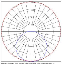
Maximum Candela = 18264 Located At Horizontal Angle = 337.5, Vertical Angle = 1.5 # 1 - Vertical Plane Through Horizontal Angles (337.5 - 157.5) (Through Max. Cd.) # 2 - Horizontal Cone Through Vertical Angle (1.5) (Through Max. Cd.)
