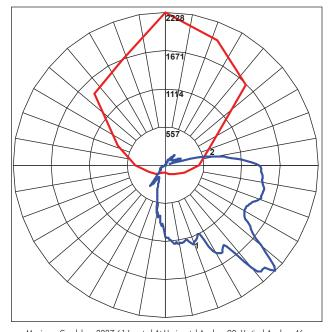
Maximum Candela = 2227.61 Located At Horizontal Angle = 90, Vertical Angle = 46 # 1 - Vertical Plane Through Horizontal Angles (90 - 270) (Through Max. Cd.) # 2 - Horizontal Cone Through Vertical Angle (46) (Through Max. Cd.)
