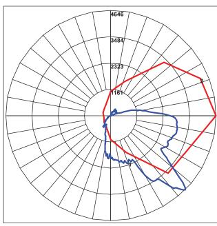
Maximum Candela = 4645.76 Located At Horizontal Angle = 0, Vertical Angle = 45 # 1 - Vertical Plane Through Horizontal Angles (0 - 180) (Through Max. Cd.) # 2 - Horizontal Cone Through Vertical Angle (45) (Through Max. Cd.)
