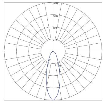
Maximum Candela = 1648 Located At Horizontal Angle = 0, Vertical Angle = 0 H - Horizontal Axial Candela V - Vertical Axial Candela
