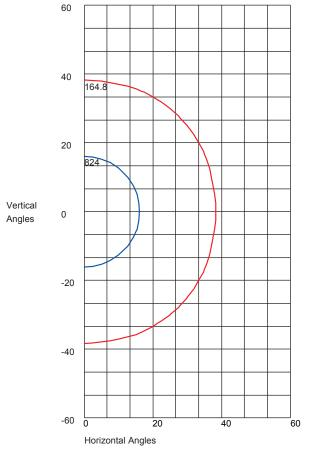
Maximum Candela = 1648 Located At Horizontal Angle = 0, Vertical Angle = 0 50% Maximum Candela = 824 10% Maximum Candela = 164.8
